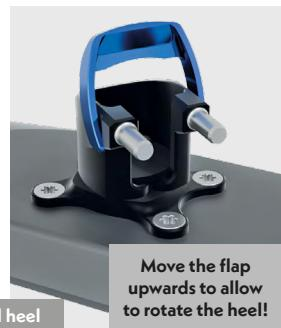
The GR Olympic binding has a swivel heel, thanks to which the ski shoe is released in the event of a fall. It is possible to turn the heel laterally to the left and to the right. The heel also releases the ski boot vertically.
